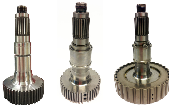
Figure 3.15: Left: weakened shaft, middle: shaft with pressed on ring, right: weakened shaft with welded ring
